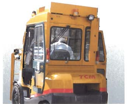
Steel cabin-enclosed type with air-cooler (available for 2-3.5ton models)
