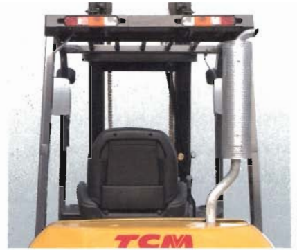
Overhead exhaust system
